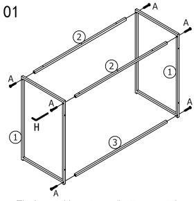
Fix 2 metal legs to top/bottom metal support tubes(2,3) with screw (A) by using hex wrench(H).
