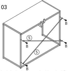
Lock the back support wire (5) on the left and right metal legs (1) with screw (B).
