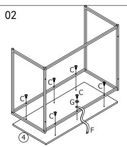
Fix assembled part "Step 01" to top panel with screw (C), fix nylon strap (F) with screw (C) and washer (G) as shown.
