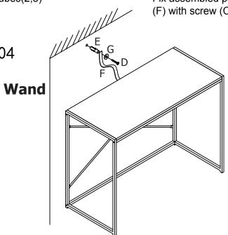
Make a hole in the right position on the wall, insert wall anchor (E) into the hole, and lock the washer (G) and nylon strip (F) on wall anchor (E) with a screw (D).
